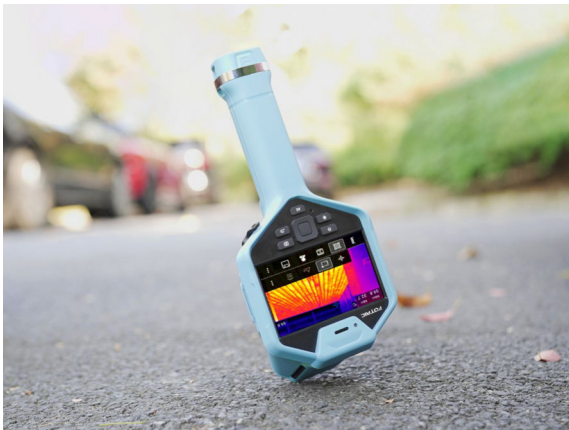
2-meter drop test
