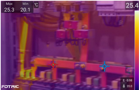
Visible light fusion thermal image (50% transparency)
